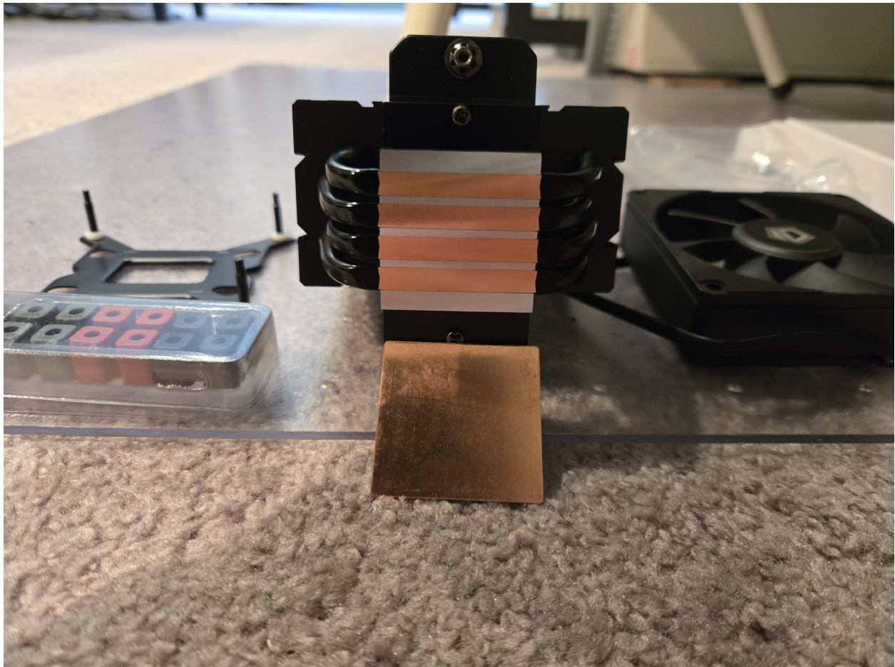
Underside of FROZN A400 Cooler, Along with Paired Copper Shim
