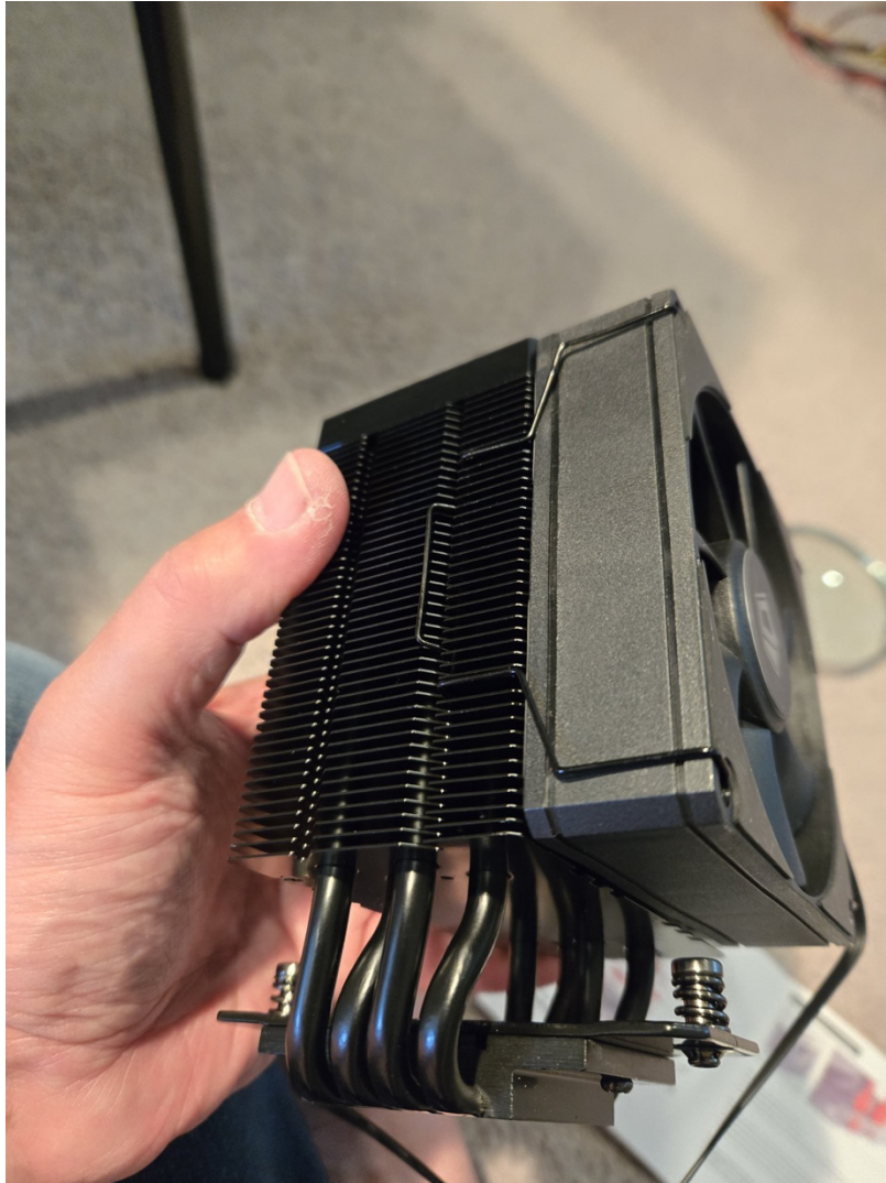
Fan Clipped to FROZN A400 Cooler
