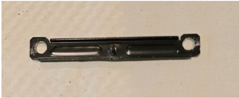
Front Mounting Bracket with Enlarged Holes
